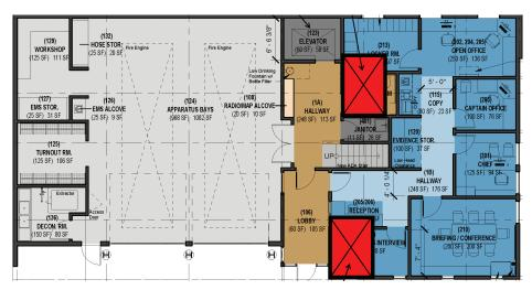
These graphics show how two possible locations for the elevator (red rectangles) would impact the Public Safety Building. On the second floor (top graphic), the elevator at the rear cuts into the firefighters' fitness room; at the front, it lands between two bedrooms. On the first floor (bottom graphic), the front elevator knocks out the police interview room, while the rear eliminates the police locker room and staff bathroom.
