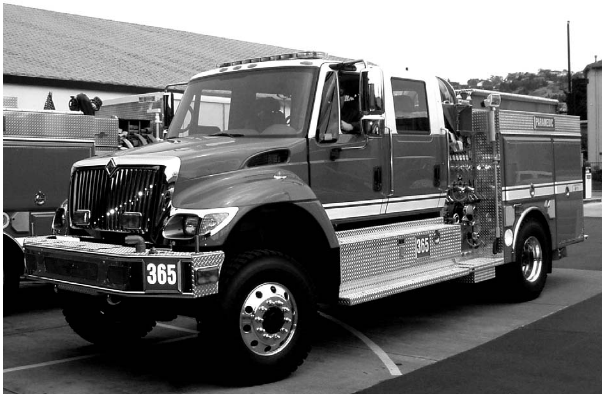
Dalmatian not included: Kensington's new custom pumper in El Cerrito waiting for firefighters to put on the final pieces of equipment. The four-wheel drive vehicle is lighter than the 21-year-old pumper it replaces and better suited to ride the hilly streets of Kensington as well as travel off-road to fight wildfires along the community's ridge.
