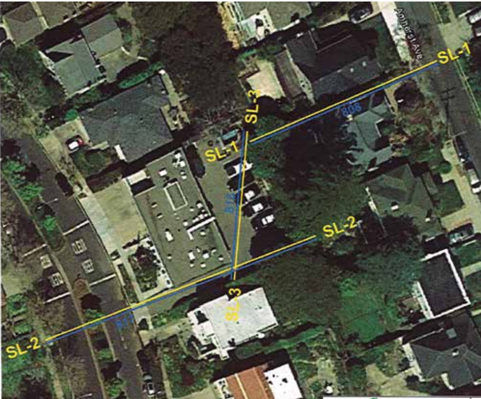
In the graphic on the left, three yellow lines trace the locations of geophones placed by Ryan Geological Consulting to sample earth layers around the Public Safety Building. The graphic above shows the composition of those layers, which are very similar along Seismic Lines (SL) 2 and 3. However, there is a marked difference in composition where SL3 intersects SL1 at the rear north corner of the parking lot behind the building, at the retaining wall. Such marked differences are assumed to indicate an active fault. A known active fault also runs along the Arlington, in front of the Public Safety Building. Graphics courtesy of the Kensington Fire Protection District.
